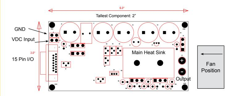
Recommended Fan: 60mm x 60mm fan with 25CFM minimum.
