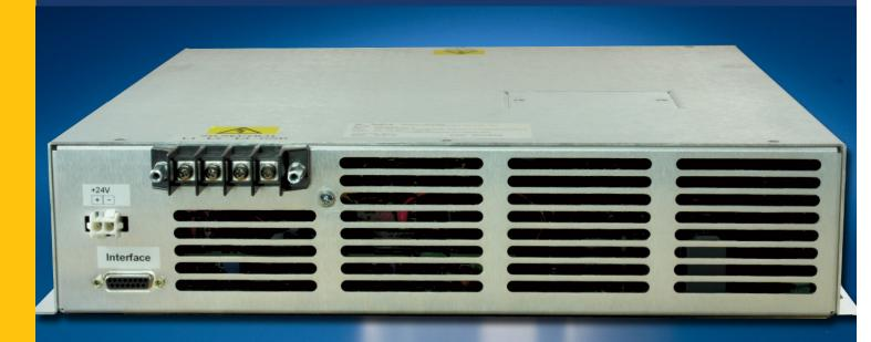
The CCHP capacitor charging power supplies utilize the latest innovations in power electronics to deliver clean and efficient energy for pulsed power applications. A high power resonant inverter ensures reliable operation in harsh environments and operating conditions. The CCHP power supply can drive traditional pulse forming networks and reservoir partial discharge circuits.
